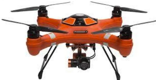
The Auto version is for when you are interested in filming and taking photos (in air and under water). The Auto version also has the added functionality of being integrated with the app, giving the options of route planning (with co-ordinates) and "follow me". This version comes out with an ULTRA HD camera which is stabilized during flight with a 2 axis gimbal.
