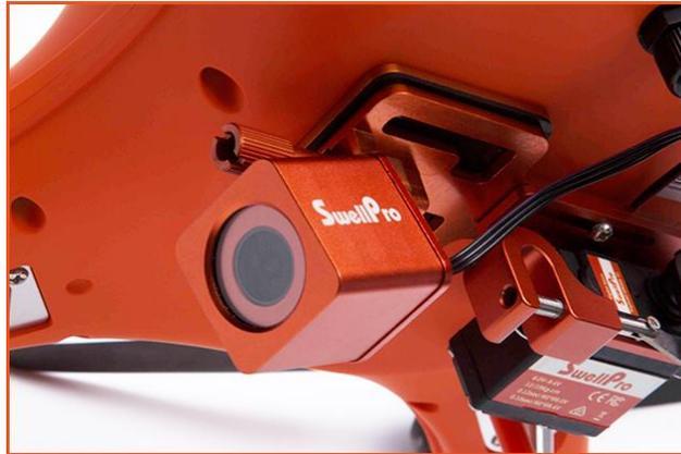
PL2 comes in the standard package of the Splash Drone 3 Fishing Edition. It is a remote payload release with an integrated, fixed-angle HD FPV camera. Set the angle of the camera before flight to suit your needs. This camera is only for live vision and cannot record video.
