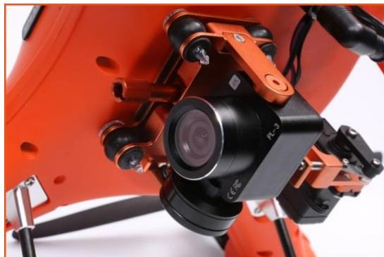
PL3 is our most advanced payload release module. The integrated, waterproof, tilt-gimballed 4K camera provides live as well as recorded video footage and allows the camera angle to be adjusted during flight. With the PL3, you can accurately locate your target drop zone and record the whole casting process in high definition
